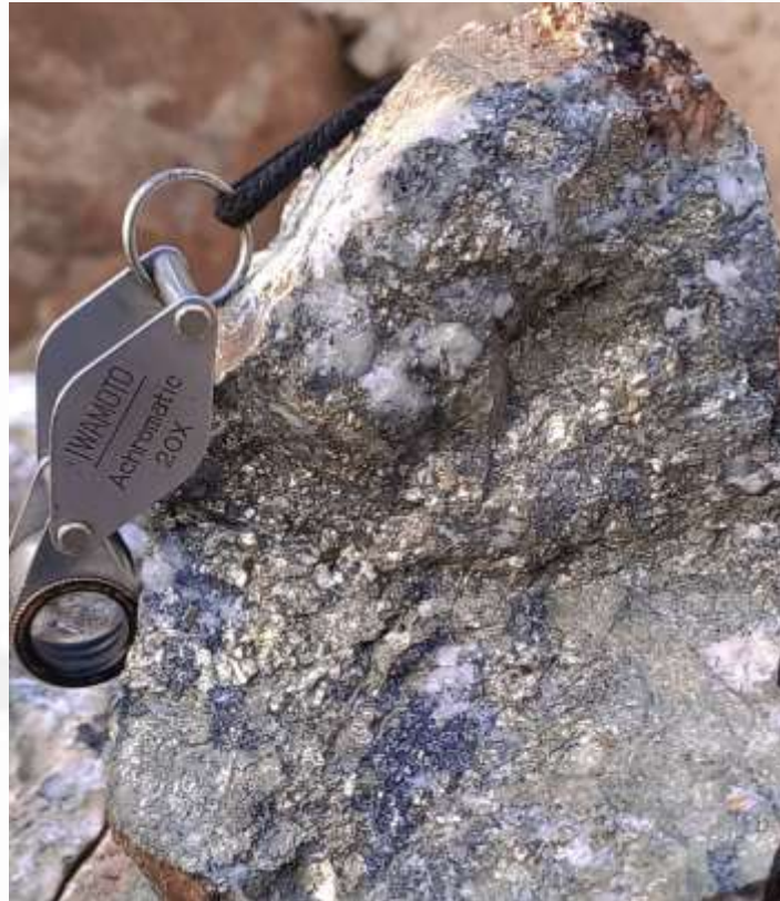
High Grade Sulphide Ore 9.69 g au/t, 13.65 oz Ag/mt and 1.00 % Cu
